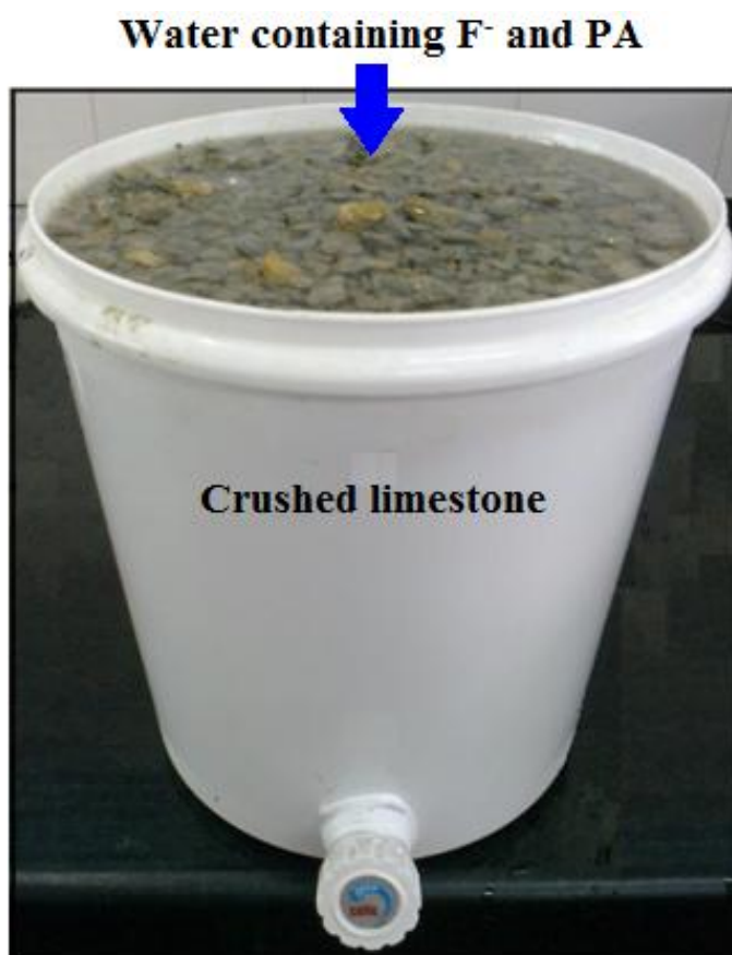
Figure 2.2. The experimental set up for laboratory-pilot experiment.
