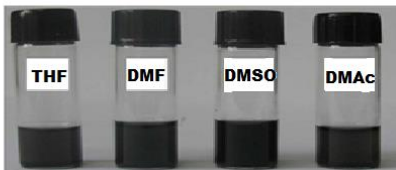
Figure 3C.1 Dispersion stability of f-RGO in different solvents after 2 months of storage
