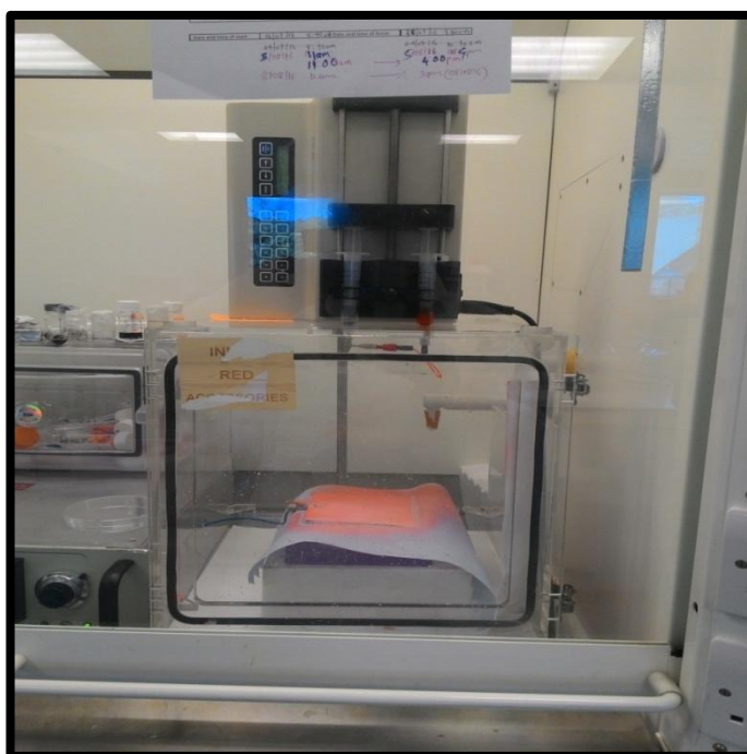
Figure 3.7. Photograph of coaxial electrospinning of MEH-PPV:PCL nanofibers.
