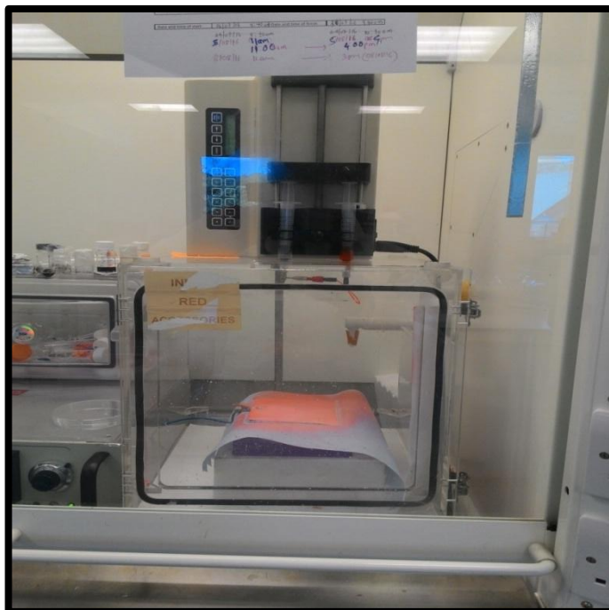
Figure 3.7. Photograph of coaxial electrospinning of MEH-PPV:PCL nanofibers.
