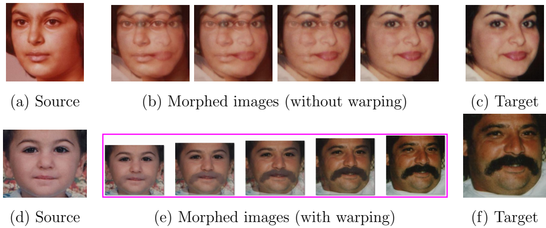
Figure 5.1: Morphing images from source to target. In first row (a) to (c), morphing without warping produces unrealistic images as facial feature points of source and target are not aligned in the morphoed images. Whether in second row (d) to (f), morphing images with warping shows a smooth transformation from source to target.
