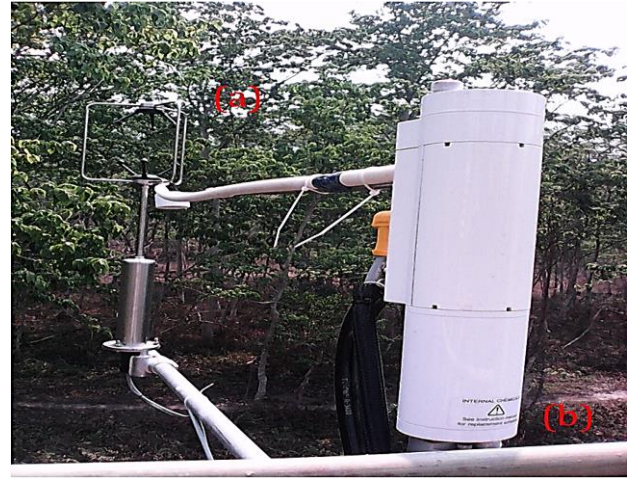
Photo 3.6: Eddy covariance system; (a) Sonic anemometer (b) LI-7200 closed path analyzer.
