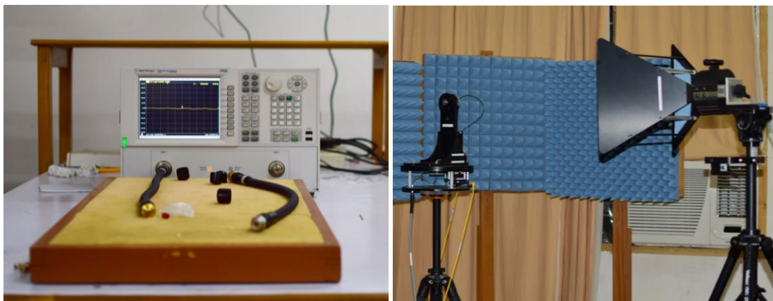
Figure 2.1 (a) Agilent VNA and (b) Antenna Measurement System showing the reference horn antenna and automated turn table for the test antenna mounting
