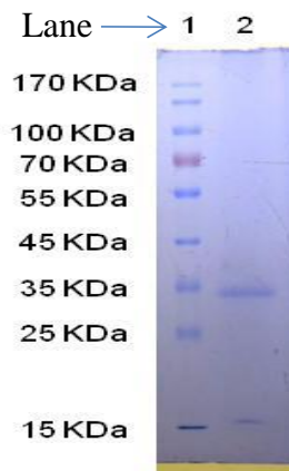
Fig. 5.1d. Determination of purity and molecular mass of AF_GF3 (lunathrombase) by 12.5% SDS-PAGE; Lane 1, protein molecular markers; lane 2, reduced lunathrombase (20.0 \mu g).
