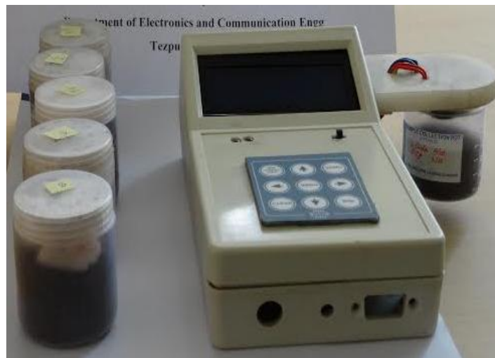
Fig. 2.31. Photograph of the handheld E-Nose system
