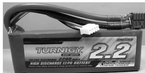
Fig. 2.24. Li-Po Battery used in the hand-held system
