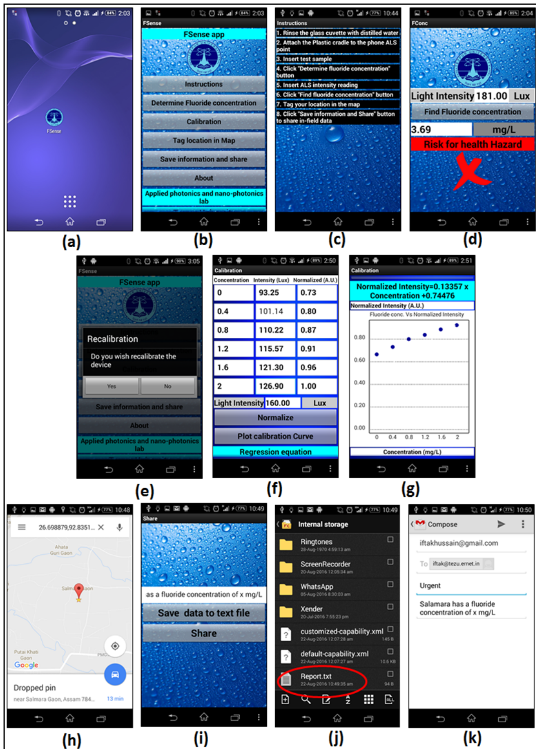
Figure 3.6: Process flow of the custom designed smartphone application.
