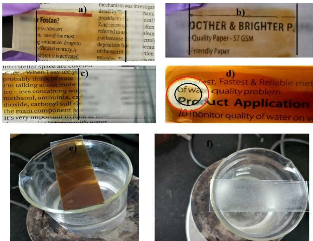
Figure 6B.11: Photos of (a, b) PCTN0.5 under 70 and 76% humidity respectively; (c) PCTN1 and (d) PCTN2.5 under 76% humidity; (e) PCTN2.5 and (f) bare glass slide over boiling water after stored at -20°C
