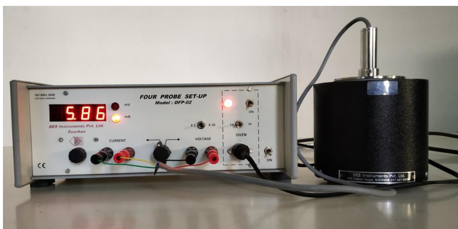
Figure 3.18: Photograph of four-probe conductivity measurement set-up (SES Instruments, Roorkee, India, model DFP-02).
