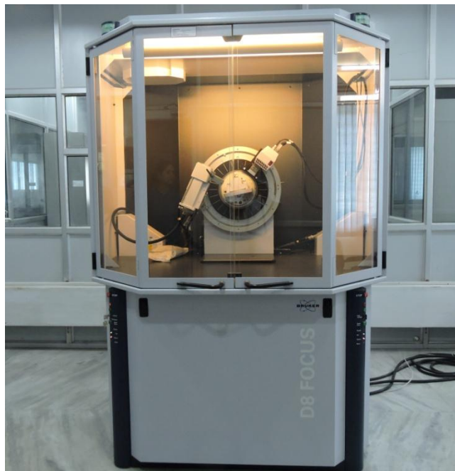
Figure 3.12: X-ray diffraction measurement unit (D8 Bruker AXS).
