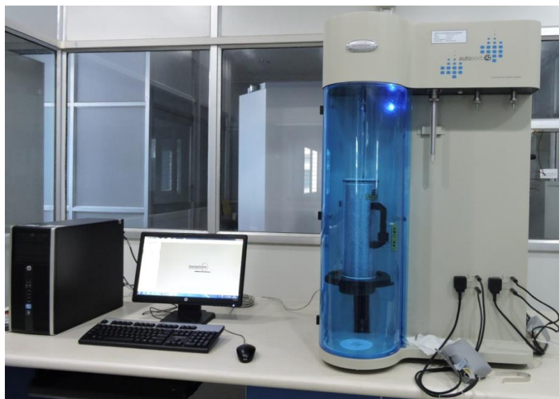
Figure 3.19: Set-up used for measurement of N_2 adsorption-desorption isotherms (Quantachrome, model NOVA 1000E).
