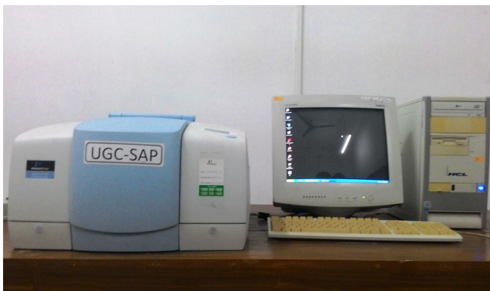
Figure 3.14: Photograph of FTIR spectrometer (Perkin Elmer, model spectrum 100).
