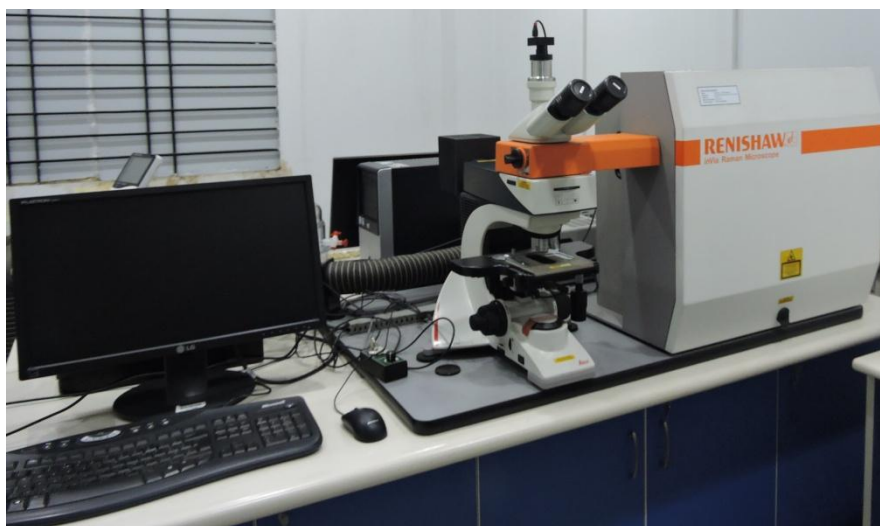
Figure 3.15: Photograph of micro-Raman spectrometer (Renishaw inVia).
