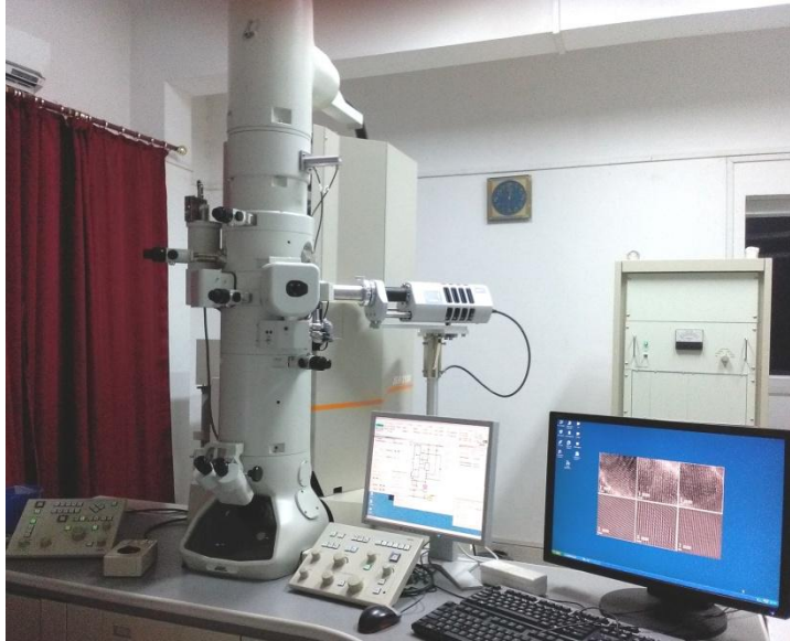
Figure 3.10: High resolution transmission electron microscope (JEOL, model JEM-2100).
