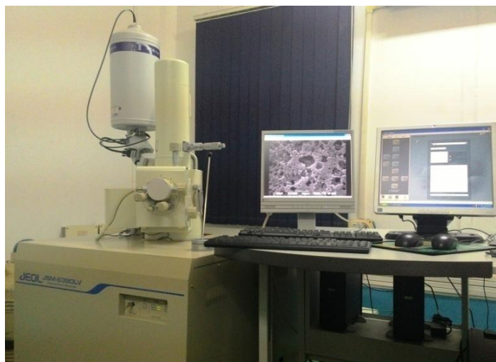
Figure 3.11: Scanning electron microscope (JEOL, model JSM-6390 LV).
