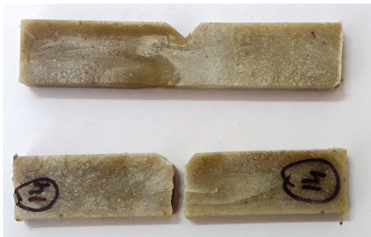
Figure 4.12: A lime sludge filled HDPE composite before and after impact test.
