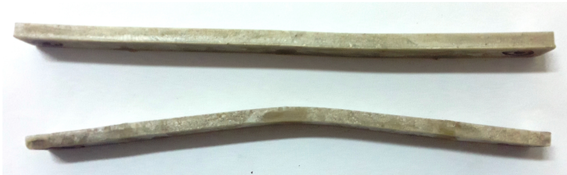
Figure 4.10: A lime sludge filled HDPE composite before and after flexural (bending) test.
