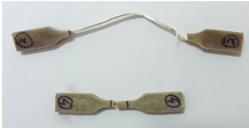
Figure 4.5: Lime sludge-HDPE composite samples after tensile test having higher and lower ductility.
