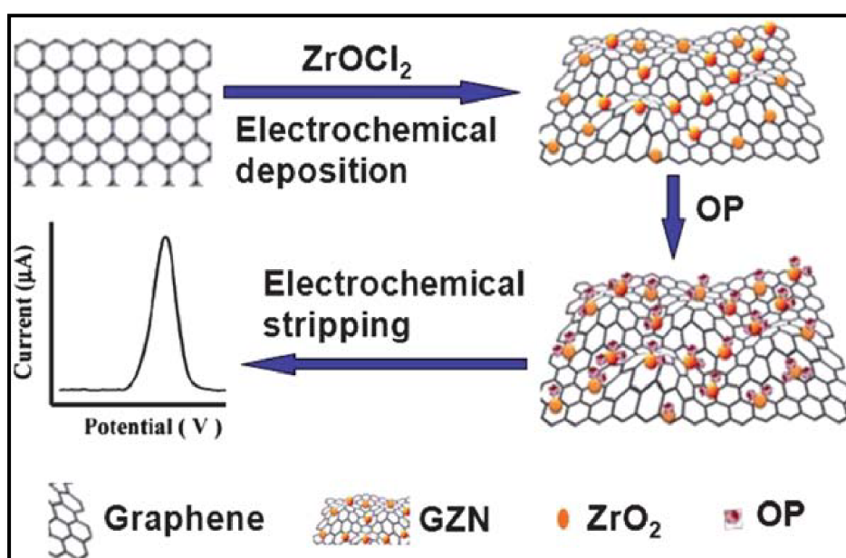
Scheme 1.2 Illustration of the one-step electro deposition of ZrO 2 -graphene nanocomposite and its application for the extraction and electrochemical detection of MP (adopted from ref. 110).
