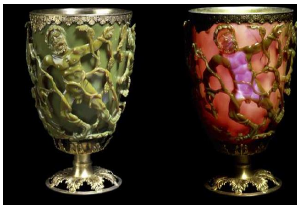
Figure 1.1: The Lycurgus cup in reflected light (left) and in transmitted light (right) [12].
