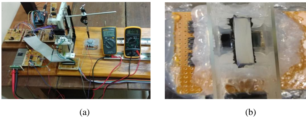
Fig. 4.2: (a) the complete measuring Setup (b) enlarged picture of a fabricated device
