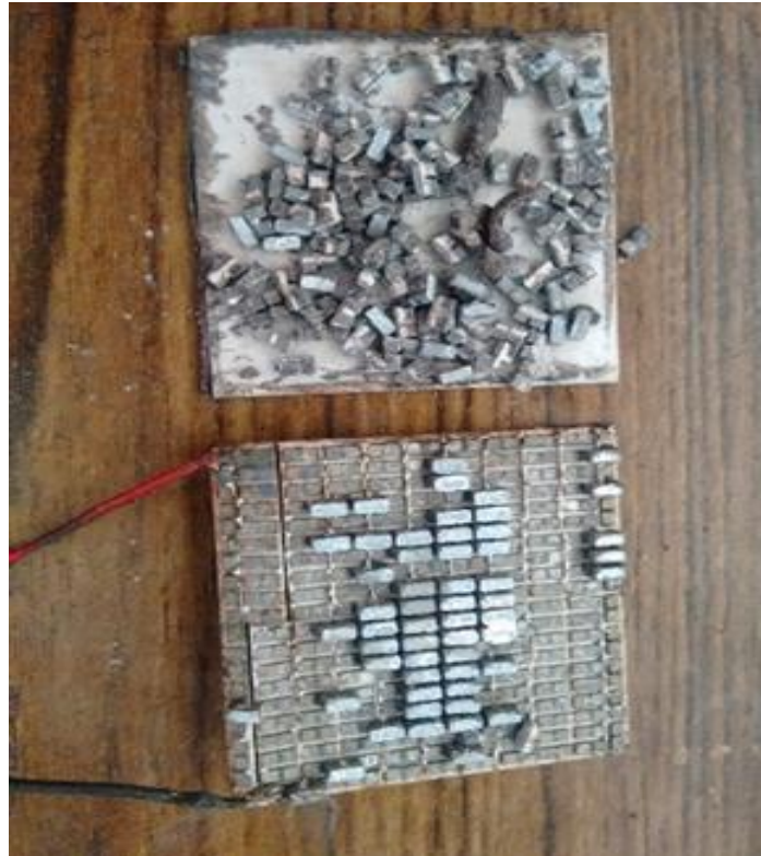
Fig. 4.18. TEG module with thermal stress at H2
