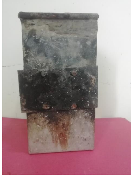
Fig. 4.9 Ash deposition on heat collector plate at H4
