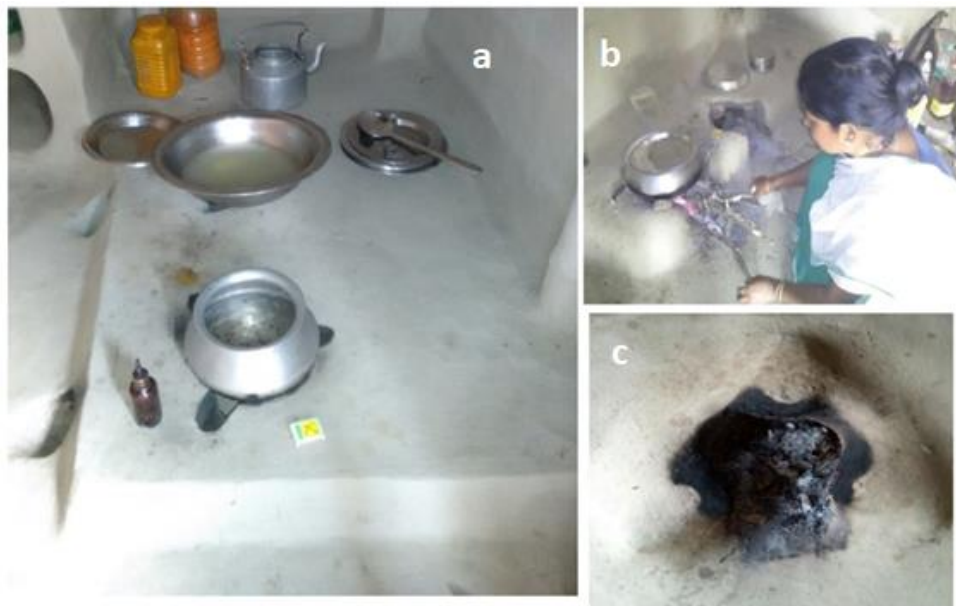
Fig. 1.1 Different versions of fixed clay stove (a) fixed clay cook stove with elevated platform, (b) cooking practice in three stone fixed clay coated cook stove, (c) three stone clay coated fixed cook stove
