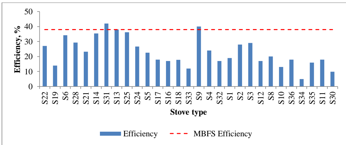
Fig. 5.4: Comparative analysis of WBT cold start results between high power stoves and MBFS [8-12]
