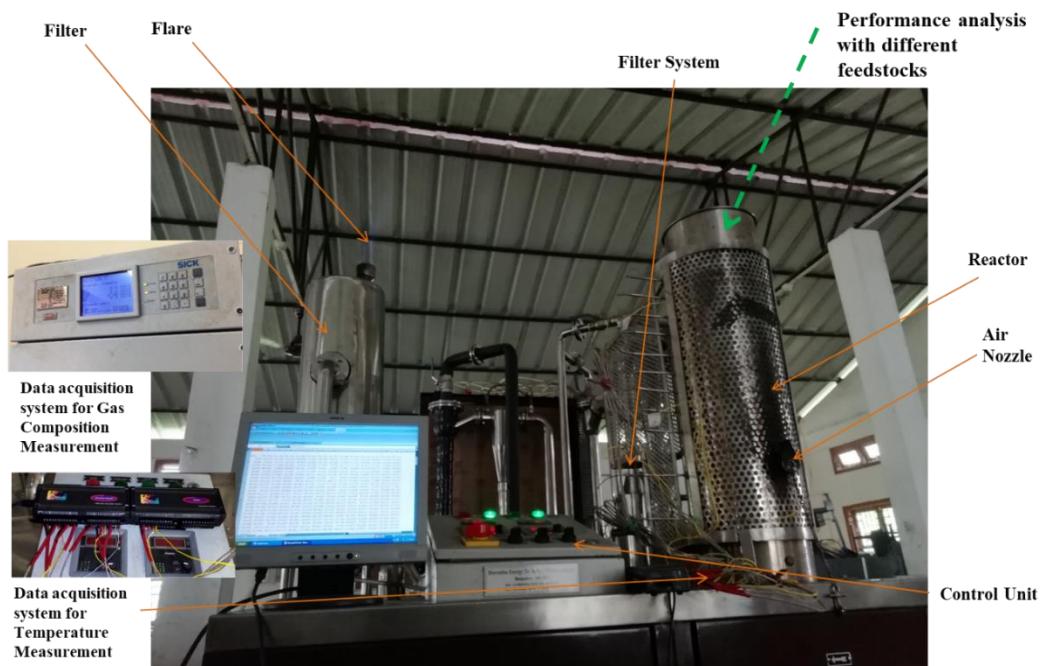
Fig. 4.9 Setup 2: 4 kW downdraft gasifier at Tezpur University, India
