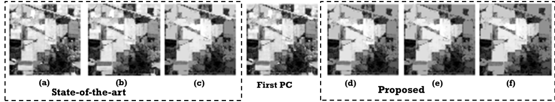
Figure 4-9: Filtered images obtained by applying the state-of-the-art and the proposed filtering method to the 1 st principal component of the Indian Pines data set by considering the area of bounding box attribute. The best filtered image obtained by the state-of-the-art method [36] considering (a) the 1 st threshold, (b) the 2 nd threshold and (c) the 3 rd threshold. The filtered image obtained by the proposed method after applying (d) the 1 st , (e) the 2 nd and (f) the 3 rd filtering operation.
