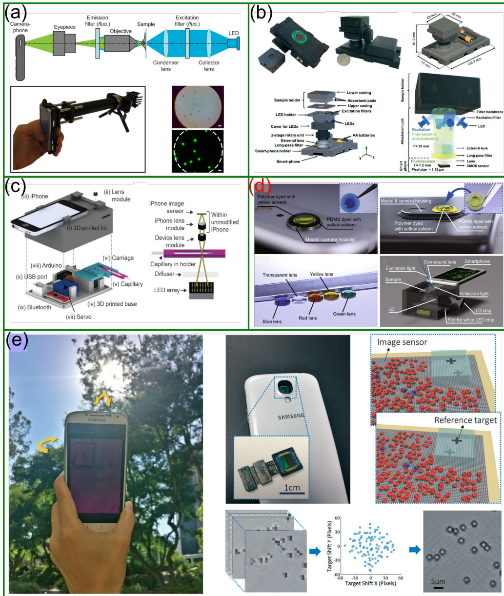
Figure 1.4: The development of different inexpensive microscopic imaging platforms on smartphone; (a) a mobile microscopy by utilizing conventional optical elements, reproduced from [26] with permission from Public Library of Science (PLOS), (b) demonstration of smartphone based fluorescent microscope for detection of water-borne parasites like giardia lamblia cysts, reproduced from [27] with permission from Royal Society of Chemistry, (c) prototype of a video microscopy on smartphone for blood-borne filarial parasites detection, reproduced from [28] with permission from American Association for the Advancement of Science, (d) demonstration of a smartphone microscope using color compound polymer lenses, reproduced from [29] with permission from Nature Publishing Group, and (e) demonstration of a chip scale lensfree microscope using ambient light, reproduced from [30] with permission from Royal Society of Chemistry.
