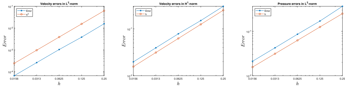
Figure 2.1: Velocity and pressure errors based on (P_2, P_0) element for Example 2.1.
