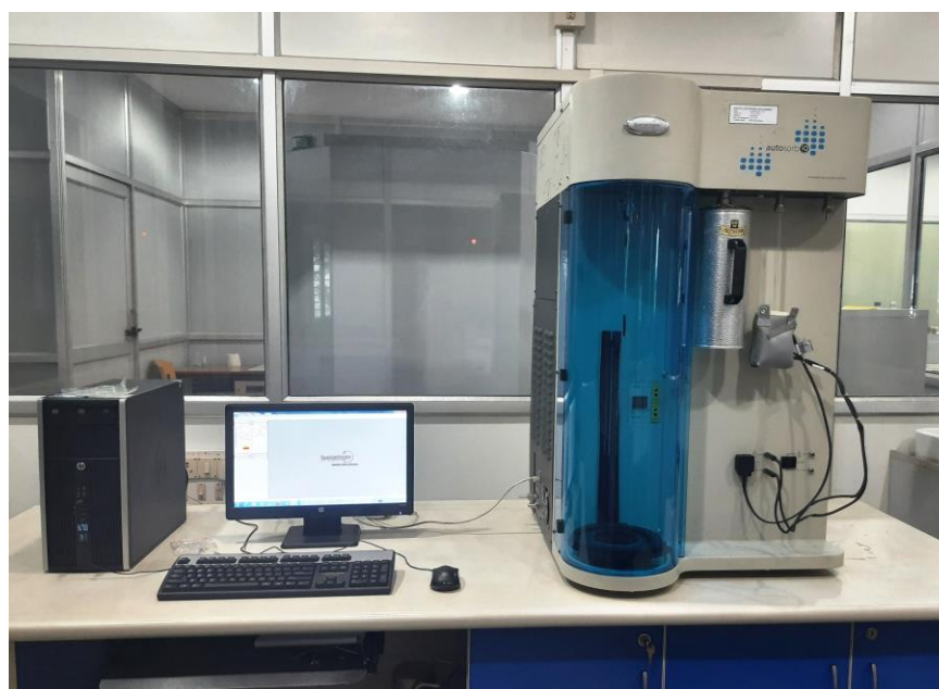
Figure 3.20: Set-up used for Nitrogen adsorption-desorption measurements (Quantachrome, model NOVA 1000E).
