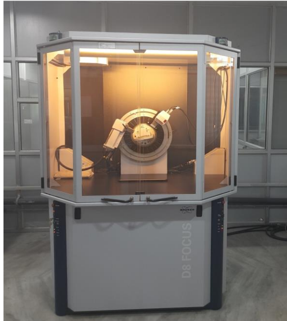
Figure 3.17: X-ray diffraction measurement unit (D8 Bruker AXS).
