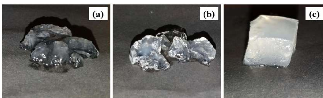
Figure 2.5. Digital photographs of hydrogels showing dimensional stability and strength of (a) SAH 1, (b) SAH 2, and (c) SAH 3.
