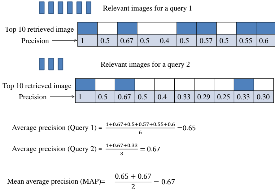
Figure. 3.12: Example computation of MAP considering two query images with different number of relevant images in dataset
