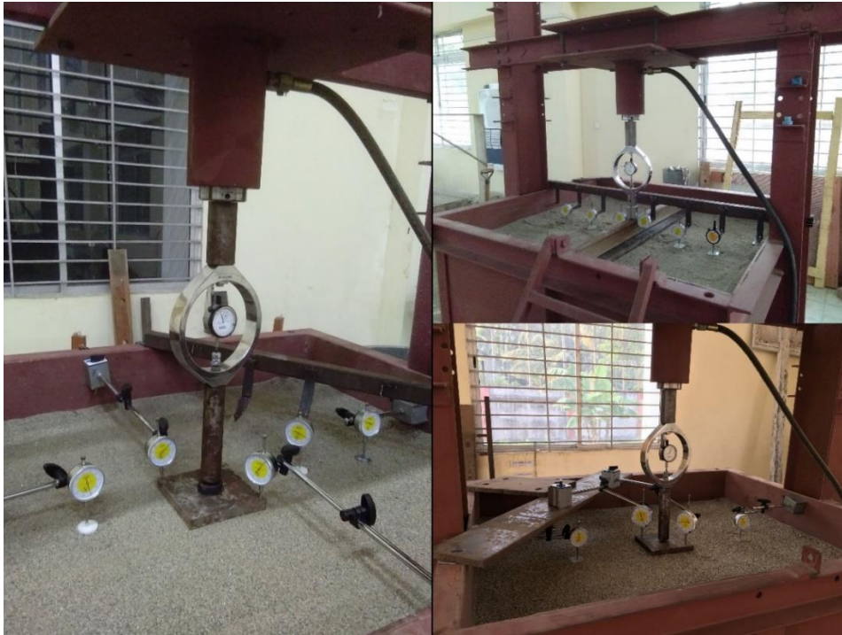
Fig. 3.15 Photograph of dial gauge arrangements for deformation measurement of the sand bed
