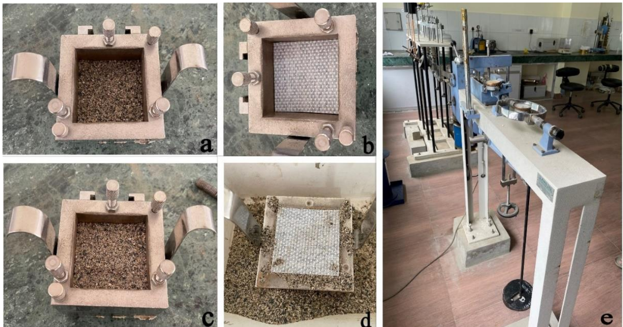
Fig. 3.9 Photographic view of (a-b-c) soil-geotextile-soil layer in the direct shear box; (d) bottom layer of soil with geotextile in the direct shear box after the test; (e) direct shear apparatus with the prepared sample.
