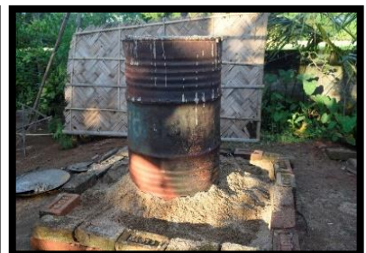
(f) Sealing off the top with metal sheet and clay
