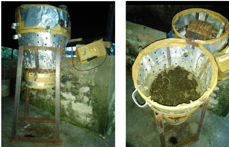
Fig 7.3.8: Mechanized with shredder and watering device incorporated vermireactors (MSVR)
