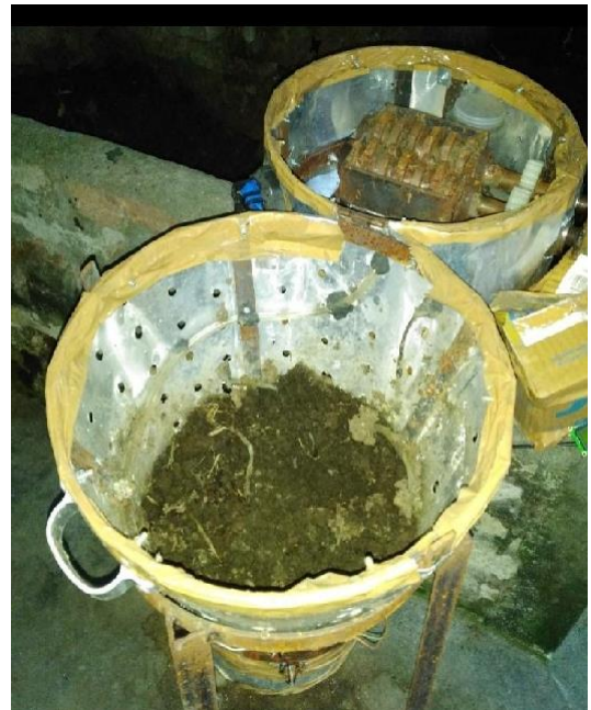
Photo4 ; Mechanized with shredder and watering device incorporated vermireactors (MSVR)
