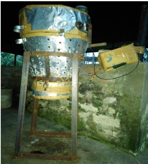
Photo4 ; Mechanized with shredder and watering device incorporated vermireactors (MSVR)
