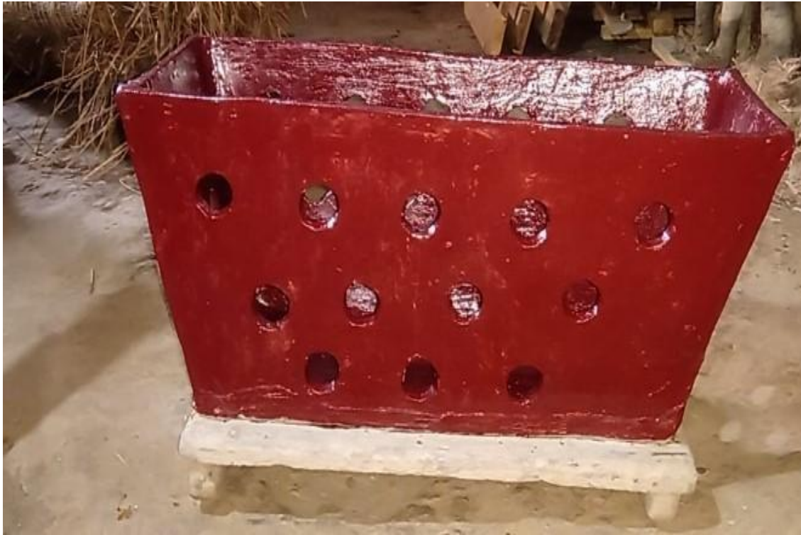
Photo3: Clay and paper paste made perforated-walled truncated cone shaped vermireactor (CPVR)
