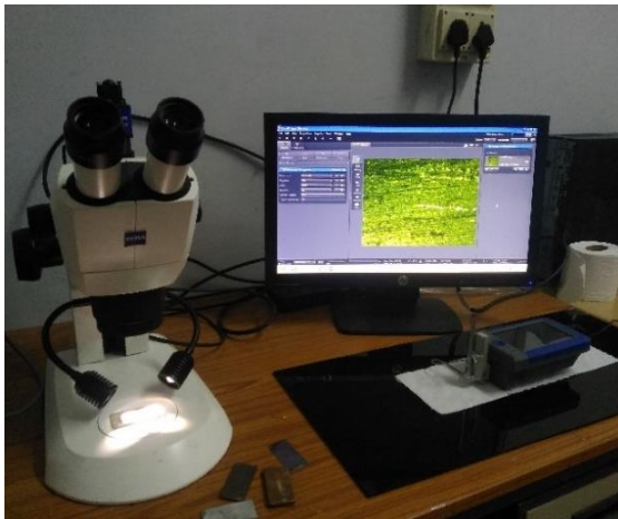
Fig. 3.4: Microscopic imaging of metal specimens with ZEISS, Stemi 305 Stereomicroscope
