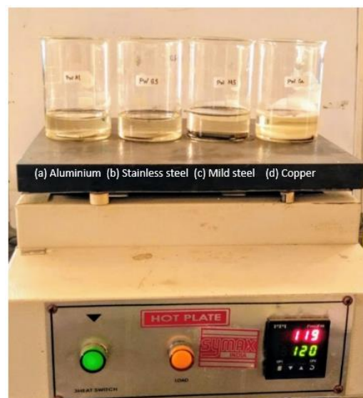
Fig. 3.2: Corrosion test of metal strips (a) aluminium (b) stainless steel (c) mild steel (d) copper with Paraffin wax up to 1000 thermal cycling test
