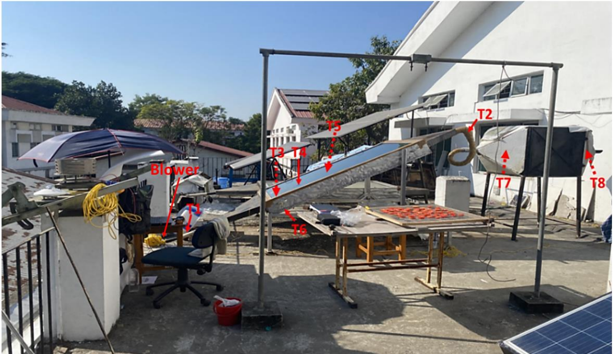
Fig. 5.2: Thermocouple locations in PCMSD
