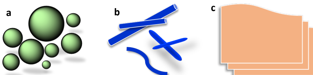
Figure 1.1. Simple representations of (a) 0-D, (b) 1-D, and (c) 2-D nanomaterials.
