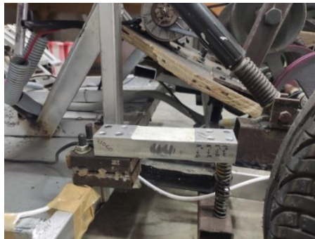
Fig.6.13 Load sensor attached to a spring in the swing arm of the EV
