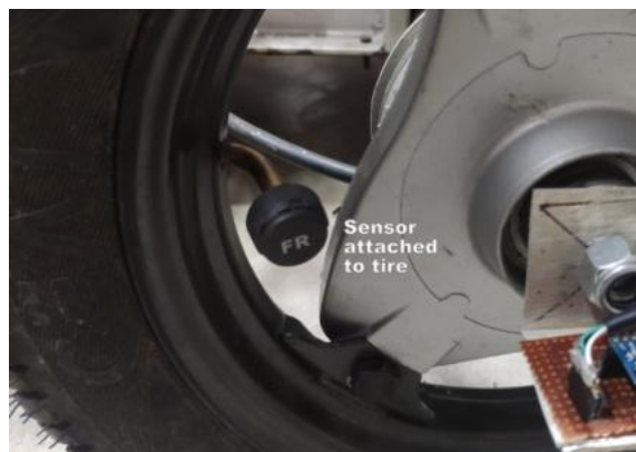
Fig.6.16 The external sensor for measurement of tyre pressure
