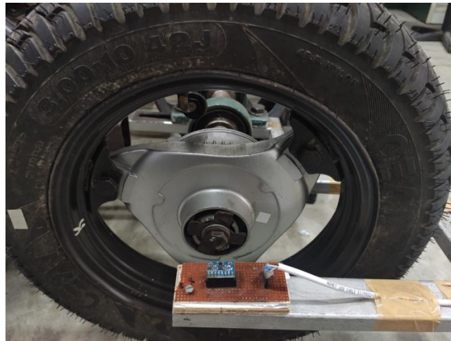
Fig.6.15 An accelerometer attached to one of the wheels
