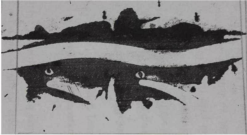
Fig.6.19 Contact patch physically determined by ink method (32psi, 60kg)
