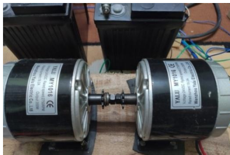
Fig.5. 21 Two motors connected along their shafts to form a motor-generator couple
