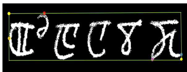
Figure 5-12: The row-wise first and last white pixels are depicted by the red and purple dots and those of column-wise are depicted by the orange and blue dots, respectively
