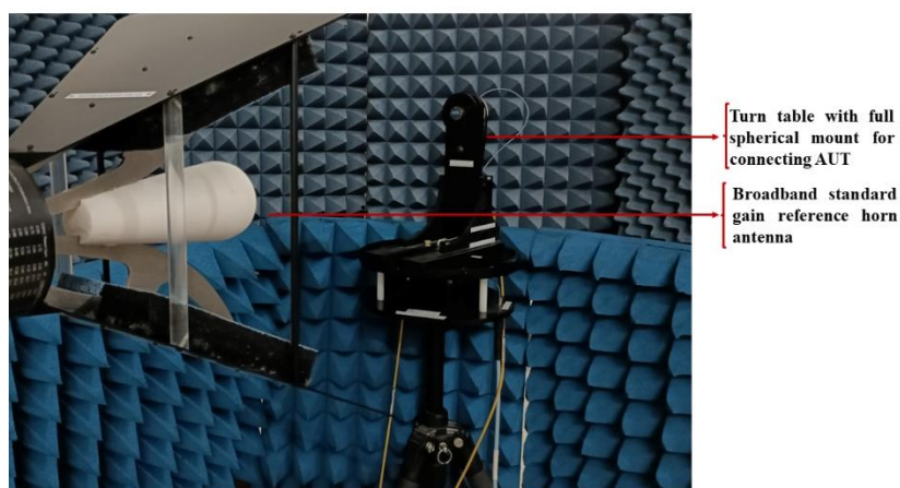
Figure 2.15 Photograph of the automated antenna measurement system from Diamond Engineering, USA (Model – DAMS 6000 with FSM)
