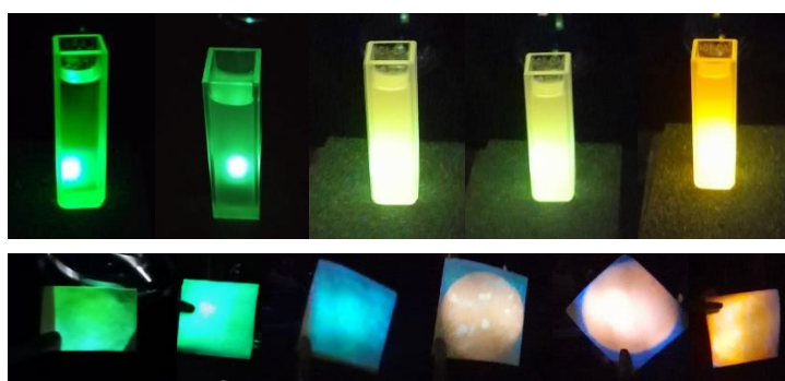
Figure 3.22: Images taken with a 365 nm UV lamp of the CPB@ZIF-8 dispersed solution (a) and coated test paper with increasing concentrations of RhB dye.
