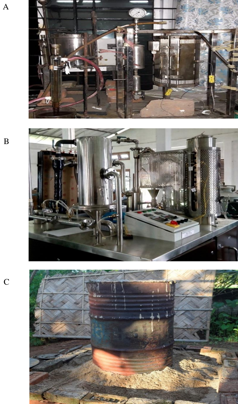
Image 3.1. Images showing (A) pyrolysis, (B) gasification and (C) conventional apparatus (kiln) used for biochar production.
