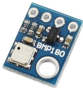
FIGURE 6.12: BMP180 sensor to measure pressure and temperature.
