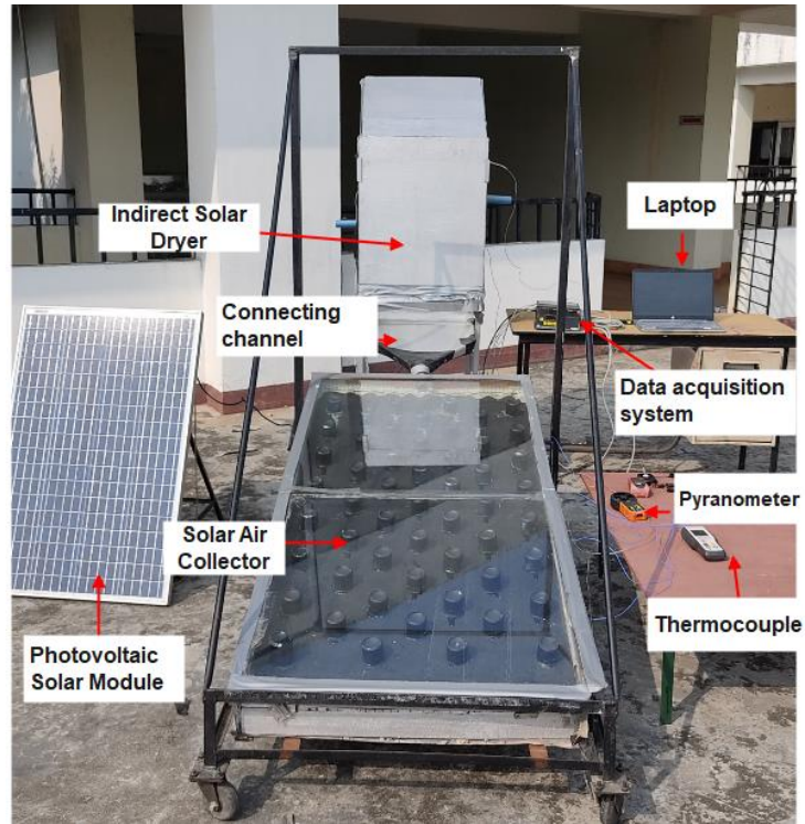
Figure 6.1 Photograph of the experimental set-up for drying of Curcuma amada .
