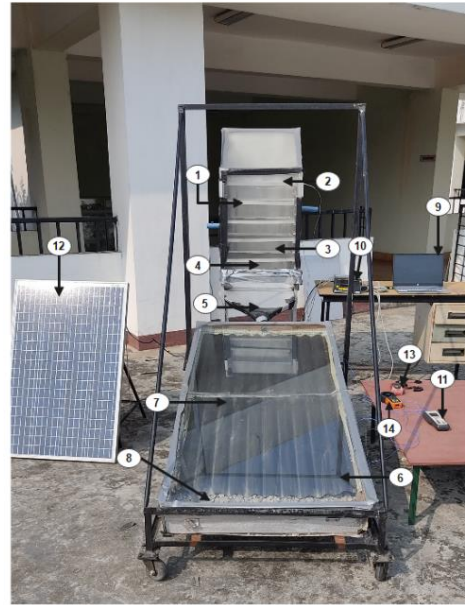
Figure 4.2 Active mixed-mode solar dryer with corrugated SAC.
