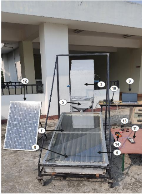
Figure 4.1 Active indirect solar dryer with corrugated SAC.
