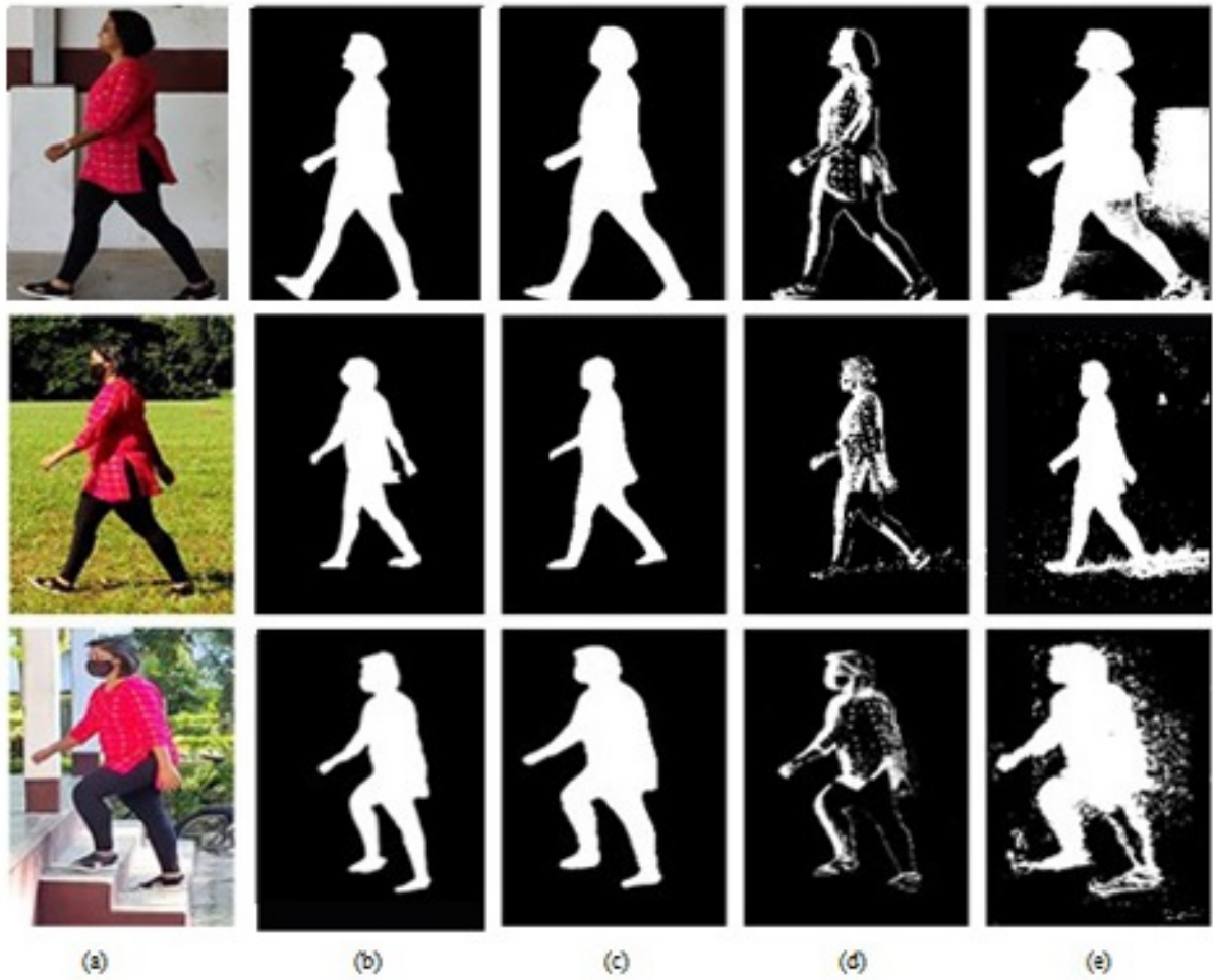
Figure 3.6: Comparison of segmentation results of the three background subtraction models for subject one.(a) Original image,(b)Ground truth,(c) DCNN ,(d) MOG2,(e) KNN
