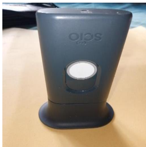
Fig. 3.2.4: NIR sensing device with sample holder
