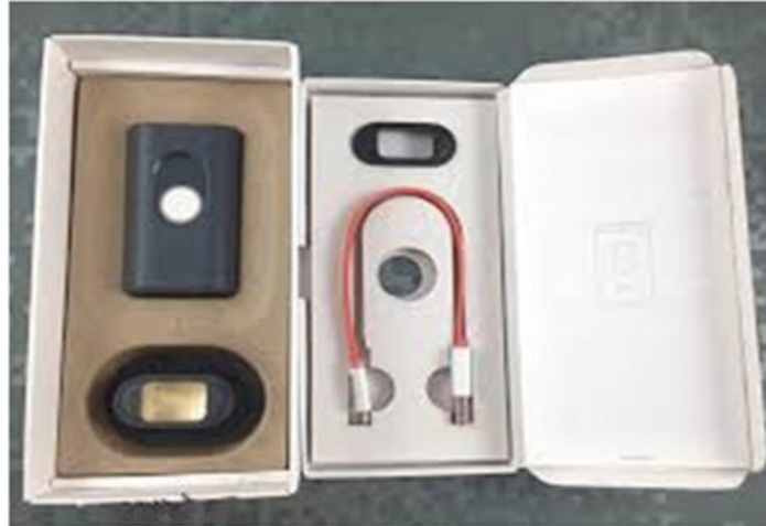
Fig. 3.2.2: Portable NIR sensing device (SCiO 1.2, Consumer Physics)
