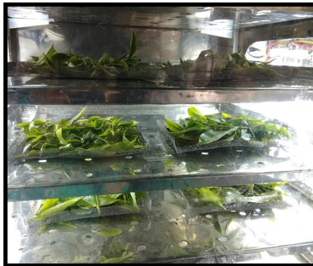
Fig. 4.2(b). Tea leaves being withered inside the EC
