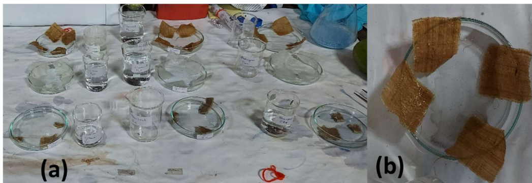
Fig 3.4: a) Rinsing of washed samples of Eri , Muga and Pat fabric b) drying procedure
