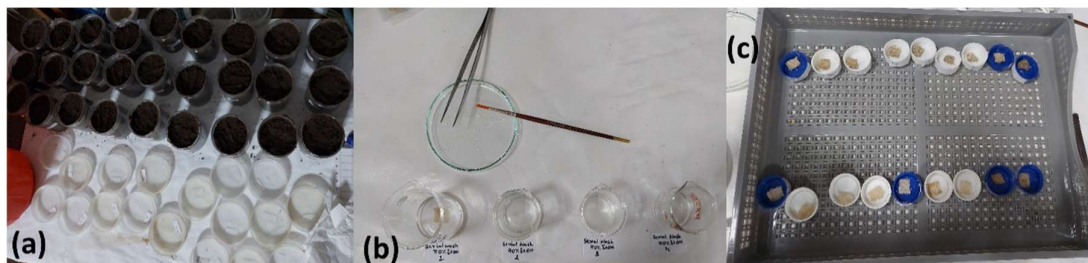
Fig 3.12: a) Phyta-jars used for soil burial b) serial washing of degraded samples c) drying of washed degraded samples
