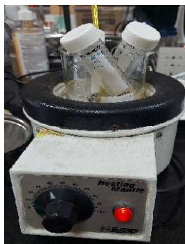
Fig 3.9: Washing of samples to check wash-fastness at 42°C
