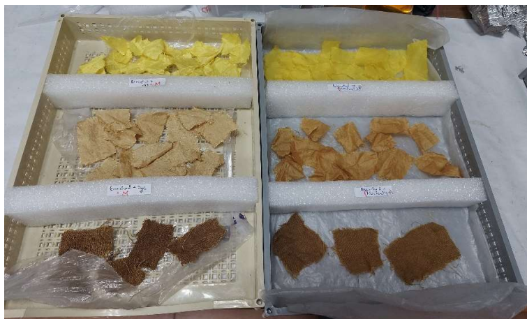
Fig 3.7: Drying method after bleaching, mordanting, and dyeing Eri , Muga , and Pat fabrics
