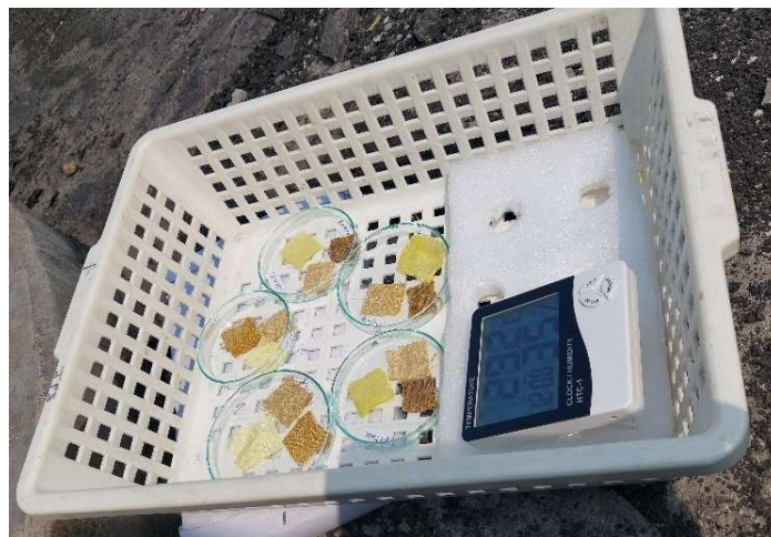
Fig 3.8: Set-up for light fastness with monitor of humidity and temperature
