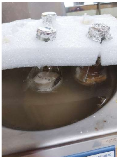
Fig 3.6: Mordant application on Eri , Muga and Pat fabric in water bath
