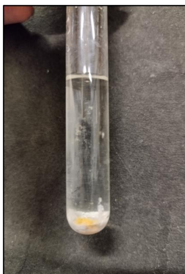
Fig. 5.23: Photographs displaying selective extraction experiments from mixture of Pb(II), Co(II), Ni(II).
