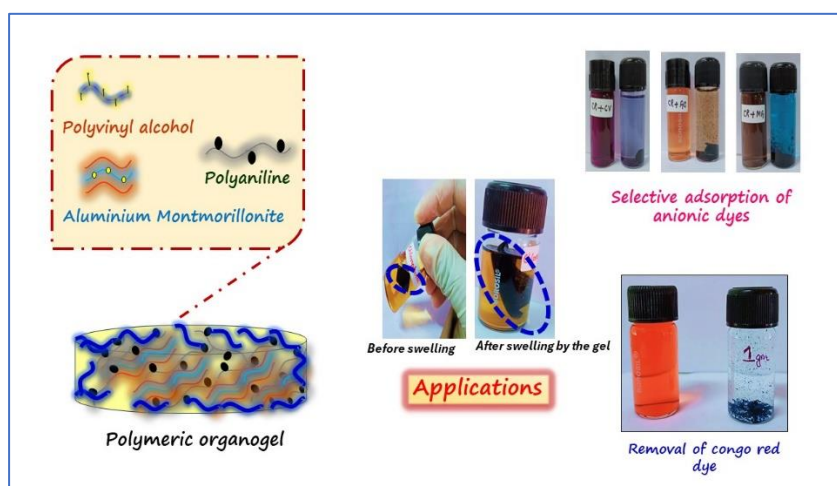
Figure4. Polymeric organogel and its application towards selective dye adsorption and phenol absorption
