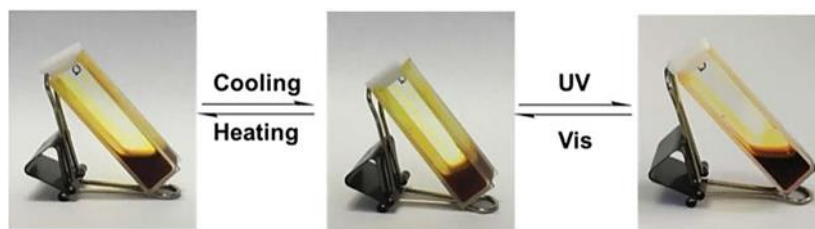
Figure 1.9 Thermal and photoresponsive property exhibited by the Azo-mLCP organogel [54]
