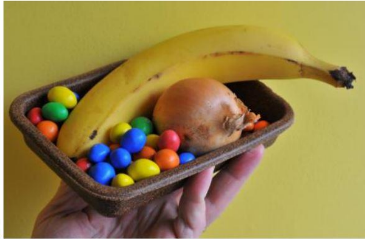
Fig. 2.8. Hot compression moulded tray from de-oiled crambe meal (adapted from Newson, 2015)
